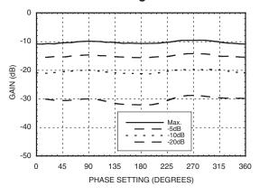
Phase vs. Phase Settings @ F= 2 GHz vs. Various Gain Settings
